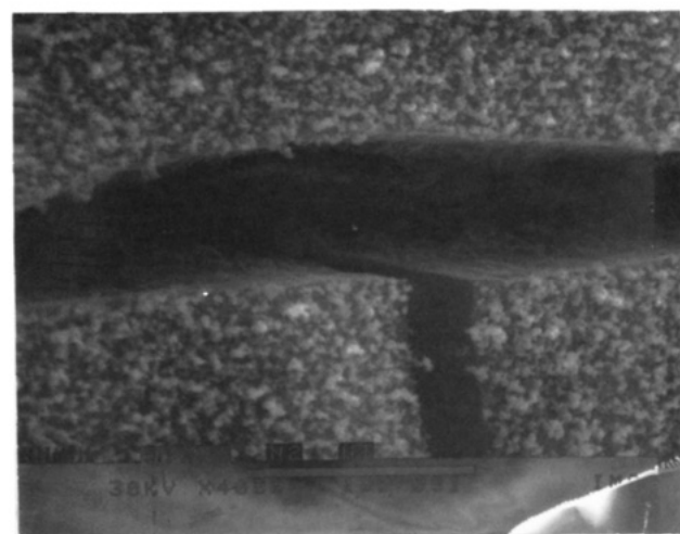
Figure 8. Cracks in structureless-type deposit formed after cooling during postthermal treatment.
