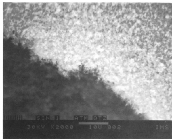
Figure 4. Structureless-type deposit, with a high density of silicon nitride particles that have settled on the surface.
